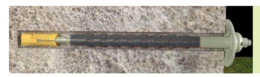
Immediate support by placement and tensioning at the tunnel face.
